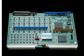
The MVME4514 Analog Scanning I/O Module is a drop-in-replacement for the GE-IP VMIC VMIVME-4514A
