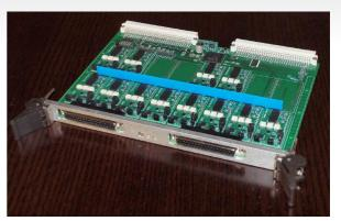
The MVME4150 is a drop-in replacement to the obsolete VMIVME-4150. It offers up to 16 optically isolated analog output channels. Each channel has its own power and ground planes that are independent of the other channels. The MVME4150 offers the following improvements over the obsolete GE-IP product.
