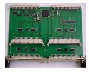
The MVME2510 64-bit TTL Digital I/O Module is a drop-in-replacement for the GE-IP VMIC VMIVME-2510B
