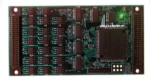
The MIPDISO Isolated Digital I/O Module is a drop-in replacement for the Acromag® IP440 and IP445 combined into one product. The customer's existing software written for these products will run the MIPDISO. The I/O connections are exactly the same.
