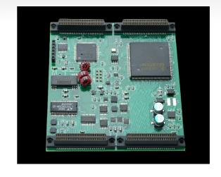
The MIPADIO is a multi-function double wide IP module offering 16 analog inputs, 4 analog outputs, and 68 digital I/O points. The unit is a drop-in replacement to the SBS IPADIO. The digital I/O section consists of 3 MC68230's programmed onto a single FPGA. Improvements over the older IPADIO include:
