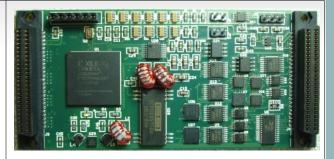
The precision A-to-D converter module provides for a drop-in-replacement to the obsolete GE-IP SBS IP-PREC-ADC.
